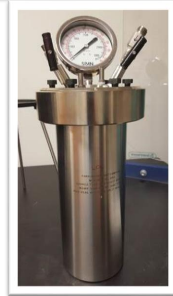
Parr Oxygen Chamber (Sample mass up to 10g)
