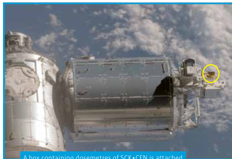
A box containing dosimeters of SCK•CEN is attached to the outside of the European COLUMBUS laboratory on the ISS. (source: ESA)
