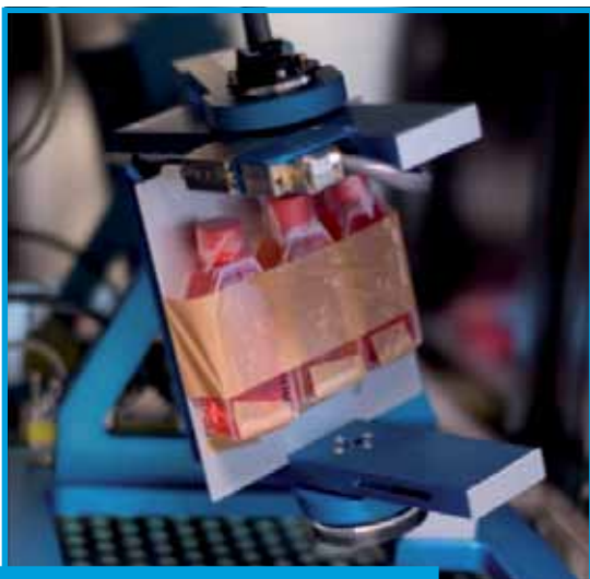
SCK•CEN device that rotates in three dimensions to simulate weightlessness.
