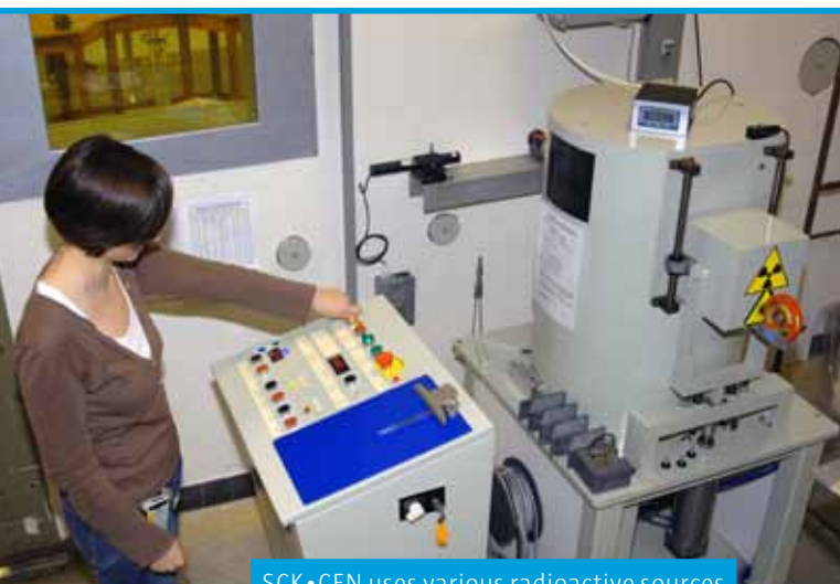
SCK•CEN uses various radioactive sources to calibrate dosimeters.
