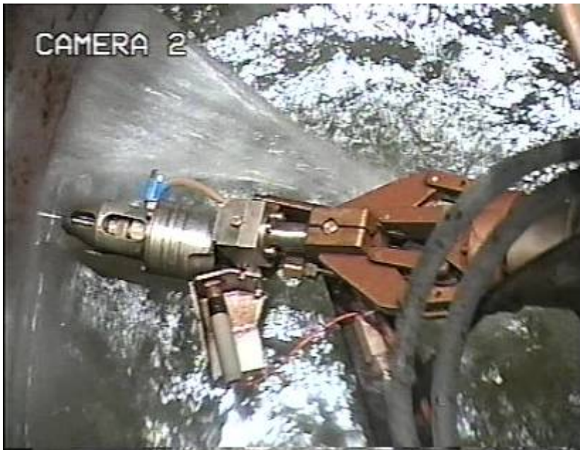
Teleoperated arm and cutting head. At the tip of the cutting head, you see the water jet cutting.
