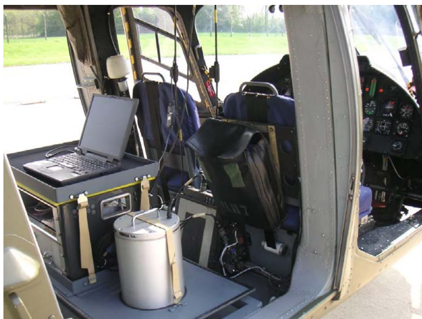
Radiation detector (cylindrical casing), analyzing electronics unit (rectangular casing) and laptop computer, mounted in the Agusta A109 helicopter, ready for use
