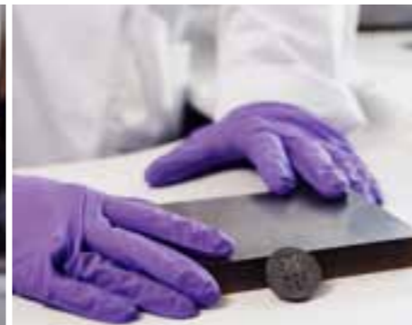
MAX phases form a material with which it is possible to make complex shapes. Conventional milling can also work perfectly.
